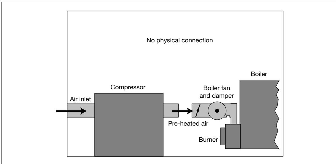
Fig 9 Indirect boiler intake of hot air
