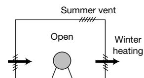
Smaller reciprocating units can also be installed so that the cooling matrix, which usually contains both coolers, is placed against an outside wall. This allows the fan to draw the coolest possible air through ventilation louvres in the wall. The air flow leaving the fan can then be directed into the building to supplement normal space heating with waste heat from the compressor during cold spells.
