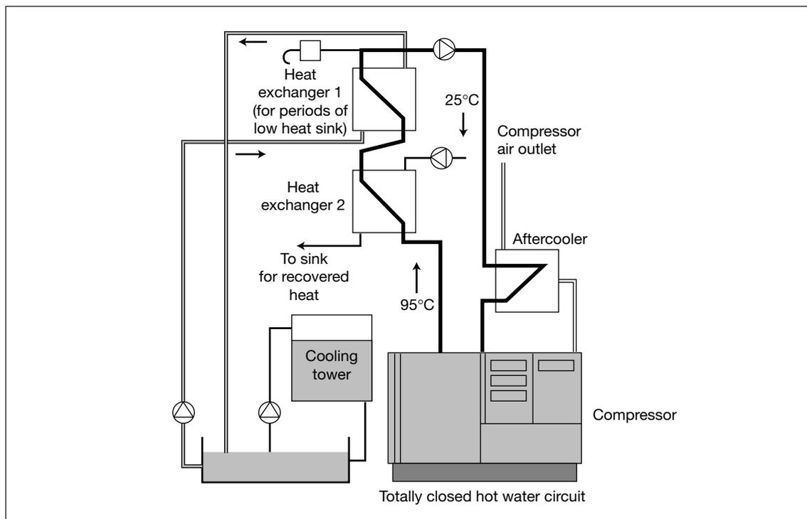
Fig 7 A sophisticated oil-to-water heat recovery system
