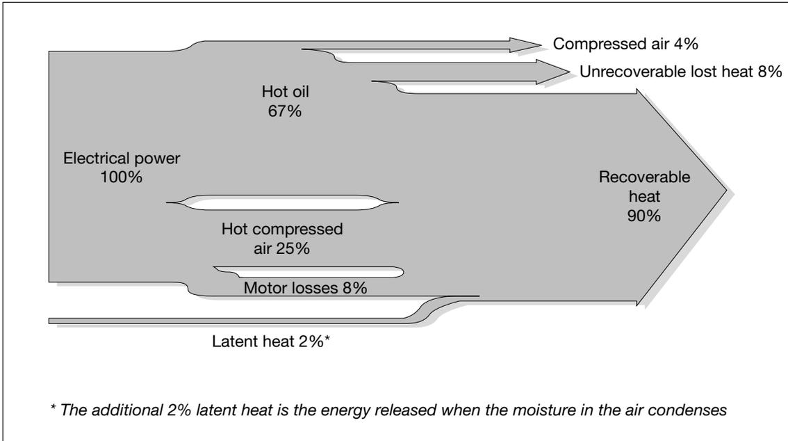
Fig 1 Energy flow in a typical oil-injected screw compressor
